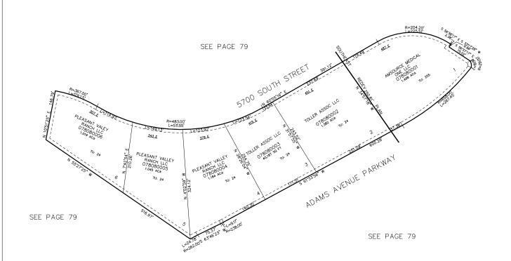
10' UTILITY & DRAINAGE EASEMENTS EACH SIDE OF PROPERTY LINES AS INDICATED BY DASHED LINES EXCEPT AS OTHERWISE SHOWN.
